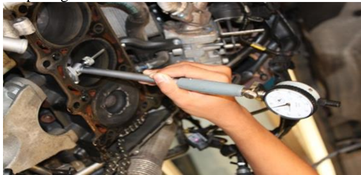
Gambar 3.2 Proses Pengukuran diameter silinder
